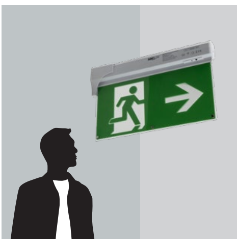
WALL SURFACE INSTALLING (FLAG TYPE)
