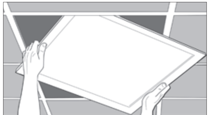
Surface installation on the modular false ceiling frame
